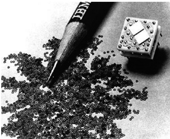
Figure 2. Magnetic core memory elements, 1955 IBM archives (VV2116) http://www-03.ibm.com/ibm/history/exhibits/vintage/images/4506VV2116.jpg
