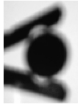
Figure 6. The diffraction fringes bordering a peg clamping a coin.
