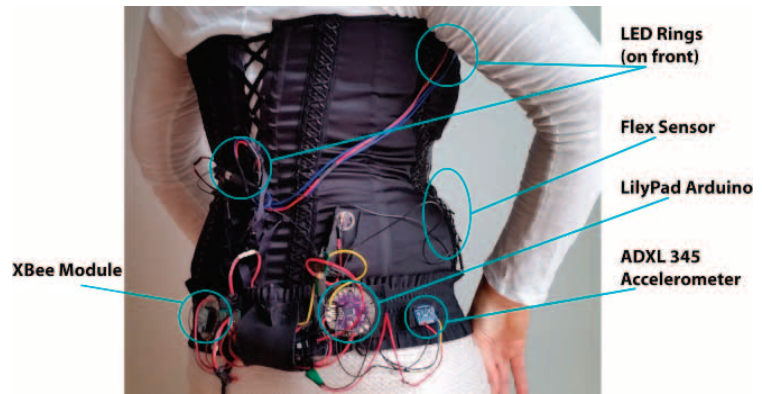
Fig. 1. Remote electroAcoustic Kinesthetic Sensing (RAKS) system, 2010. (© Steven Kemper)
