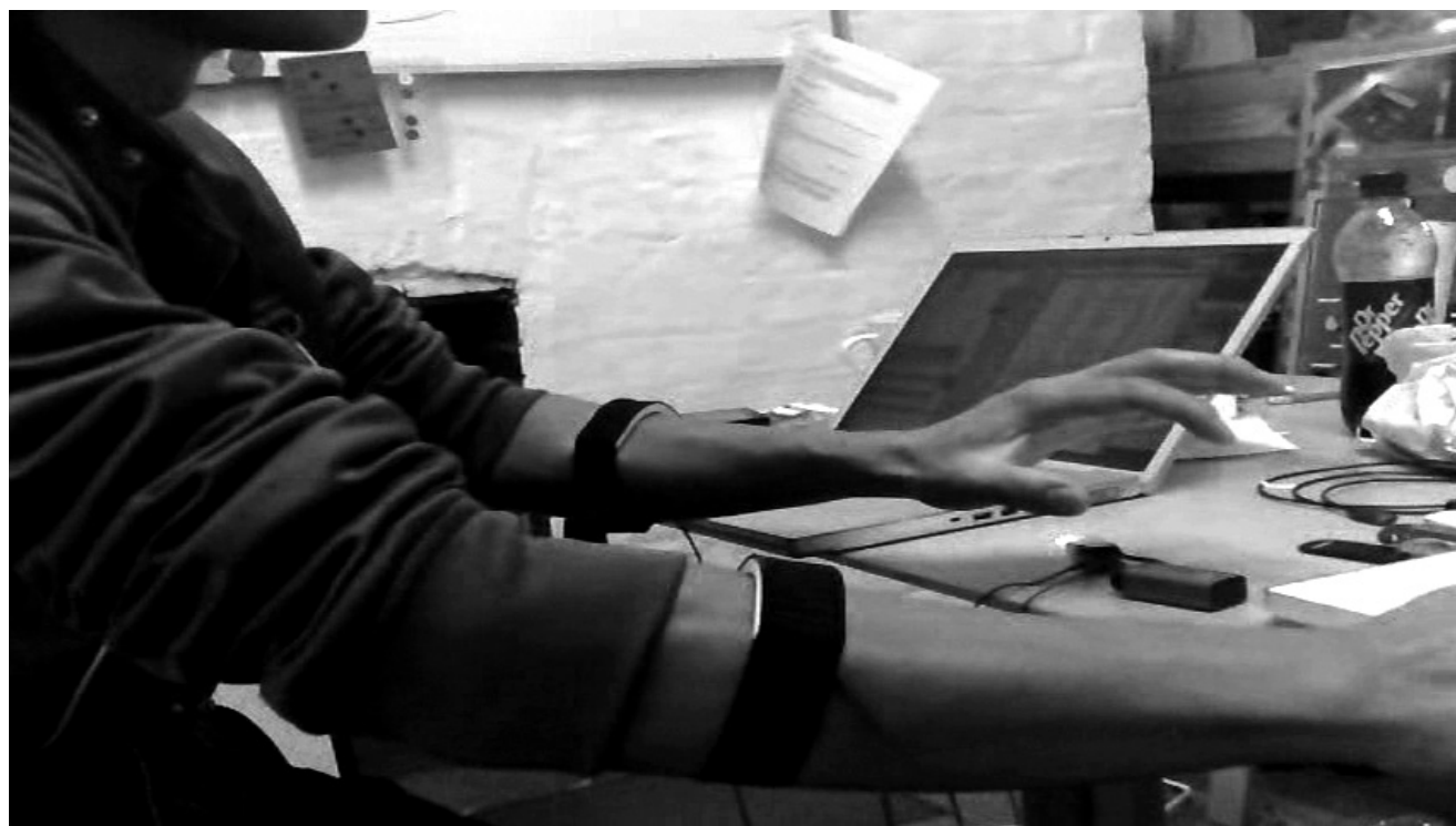
Fig. 3. Atau Tanaka wearing the EMG sensors in the positions we used. (Photo © Sarah Nicolls)
