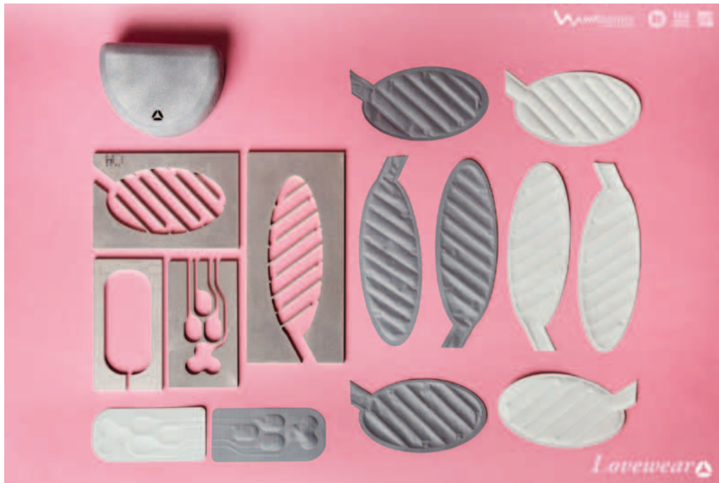
Fig. 7. Final lamination tools and sample produced. (© Emanuela Corti and Ivan Parati. Photo: Raoul XV.)
