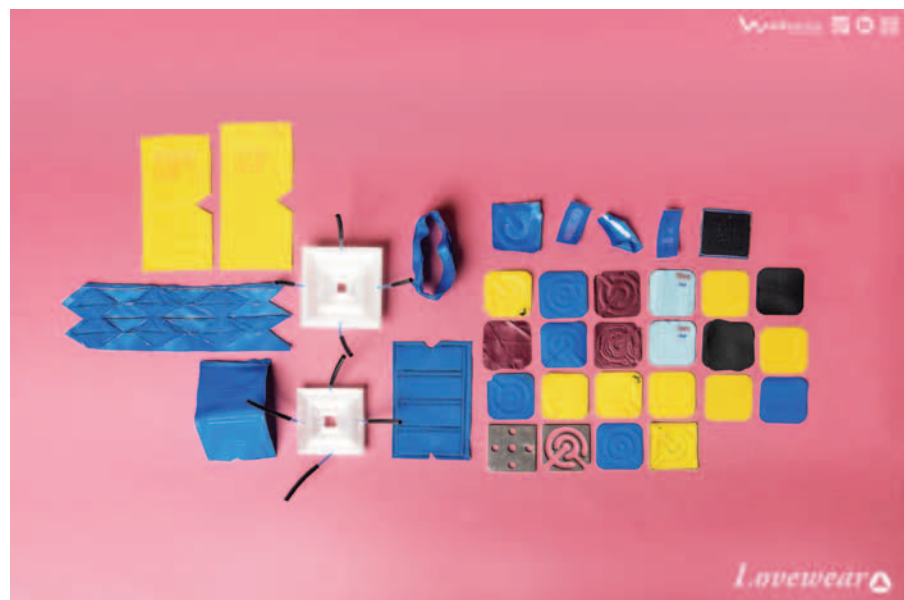
Fig. 6. Welding tests. Various shapes and structures have been considered to support pressure and movement. (© Emanuela Corti and Ivan Parati. Photo: Raoul XV.)
