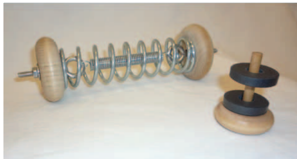
Fig. 3. Schematics and examples, respectively, of objects made up of two "particles" and C/T force components exhibiting a "simplest tensegrity" (see notes 5 and 20). Compression as lines (-) and tension as dashes (- -). (© J. David Van Horn)
