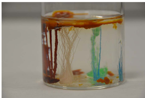
Figure 1. Plantlike structures: a classical chemical-garden experiment.
