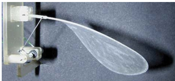
Figure 7. Flash photo showing deflection while flapping.
