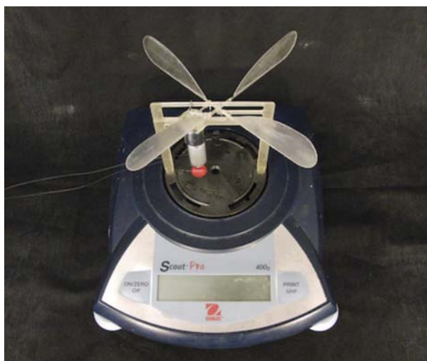
Figure 12. Four-wing test stand precisely replicating the geometry and kinematics of the real ornithopter fuselage for the purpose of characterizing lift and power performance of the four-wing configuration.
