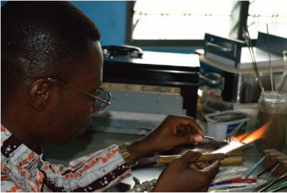
30 Cedi Djaba creating a bead with imported glass canes and lampwork beadmaking techniques, Cedi Beads Industry, Odumase Krobo, Ghana. 2013.
